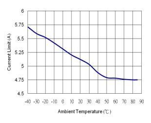
Figure 8. Current Limit vs. Temperature
