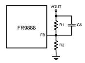
For optimizing the feedforward capacitor, knowing the cross frequency is the first thing. The cross frequency (or the converter bandwidth) can be determined by using a network analyzer. When getting the cross frequency with no feedforward capacitor identified, the value of feedforward capacitor C6 can be calculated with the following equation:
