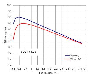
Figure 5. Efficiency vs. Load Current
