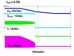
Figure 16. Power Off through VIN Waveform
