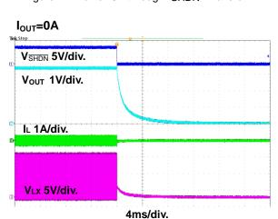
Figure 19. Power Off through SHDN Waveform
