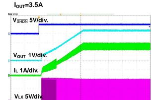
Figure 18. Power On through SHDN Waveform
