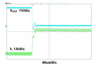
Figure 22. Short Circuit Test
