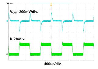
Figure 21. Load Transient Waveform
