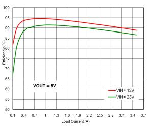
Figure 7. Efficiency vs. Load Current
