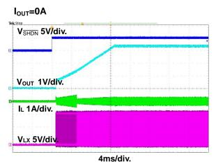
Figure 17. Power On through SHDN Waveform
