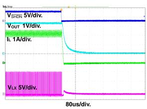
Figure 20. Power Off through SHDN Waveform
