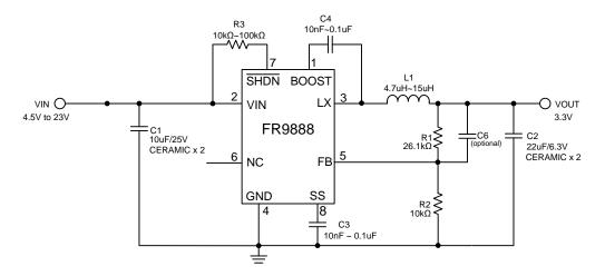
Figure 2.  $C_{\text{IN}}/C_{\text{OUT}}$  use Ceramic Capacitors Application Circuit
