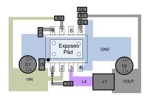
Figure 23. FR9888 SOP-8(Exposed Pad) package C<sub>IN</sub>/<sub>COUT</sub> with EC capacitors Recommended PCB Layout Diagram
