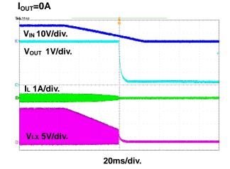
Figure 15. Power Off through VIN Waveform
