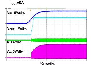
Figure 13. Power On through VIN Waveform
