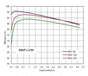
Figure 6. Efficiency vs. Load Current
