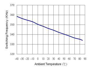
Figure 10. Switching Frequency vs. Temperature
