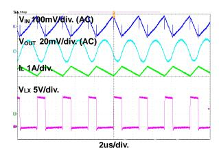
Figure 12. Steady State Waveform
