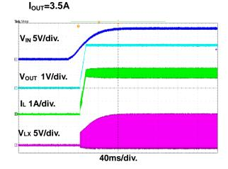
Figure 14. Power On through VIN Waveform
