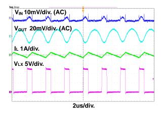
Figure 11. Steady State Waveform
