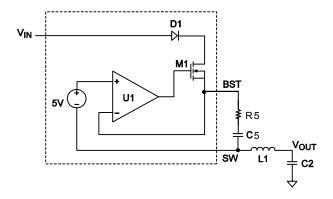
Figure 3—Internal Bootstrap Charging Circuit Startup and Shutdown
