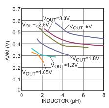
Figure 6— AAM Selection for Common Output Voltages (V<sub>IN</sub>=4.5V-24V)
