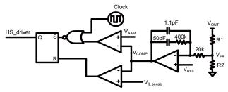
Figure 2: Simplified AAM Control Logic
