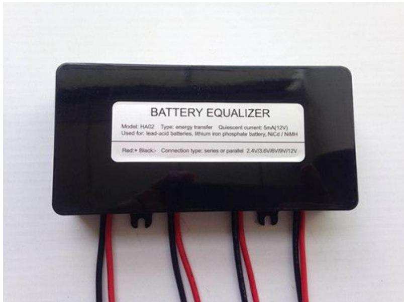
BT02 battery equalizer is energy transfer type equalizer, it can compensate for batteries with two sides. The equalizer starts to work when there are 10mV between two batteries. The current will flow from a higher voltage to low voltage, eventually reach equilibrium. It can connect with battery system with 24 hours , to keep the system energy balance automatically, no need manual maintenance.
