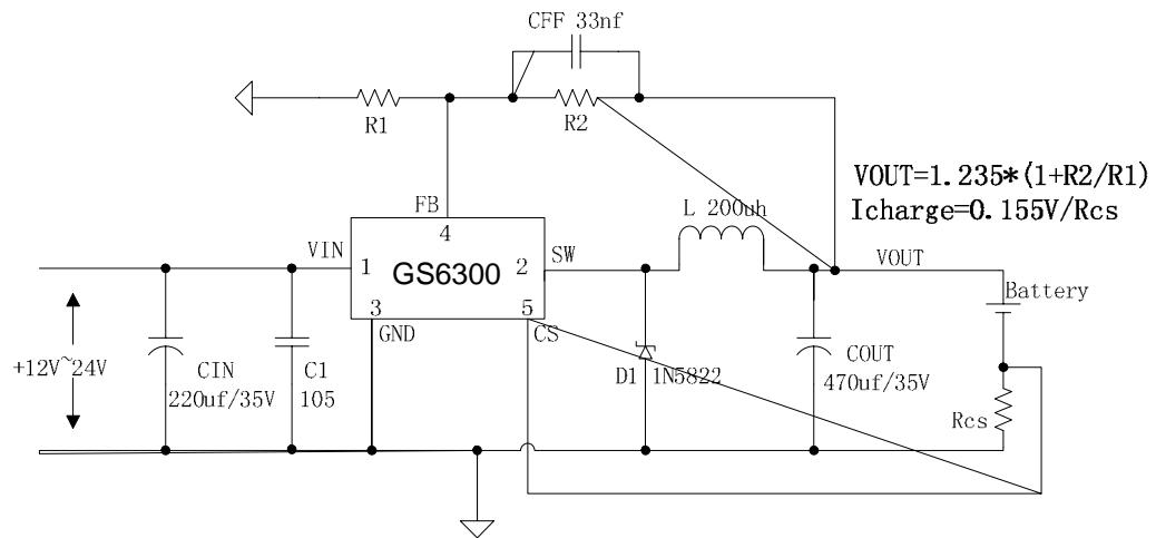
Figure4. GS6300 Typical Application Circuit (Li Battery Charger)
